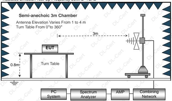
(C) Radiated Emission Test-Up Frequency Above 1GHz
