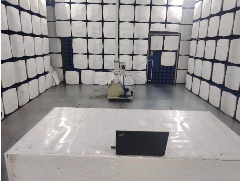
Radiated emission test view
