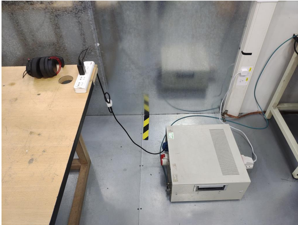
Conducted Emission Test Setup:
