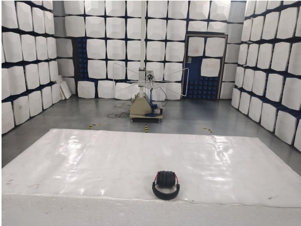
Radiated Emission Test Setup:
