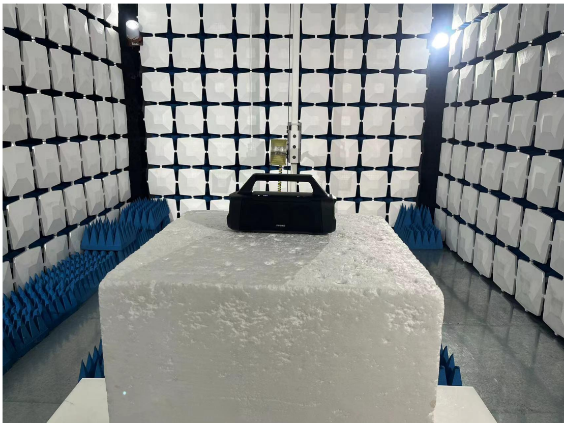
Above 1GHz for radiated emission test setup
