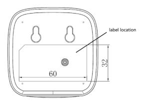
The label is printed to the back of the device with ink.
