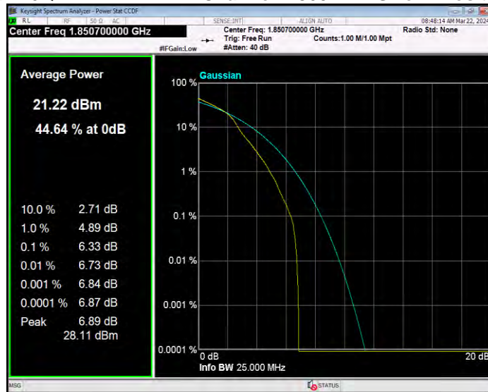
Band2 16QAM BW=1.4MHz Channel=18900 RB Size=1 Position=#0
