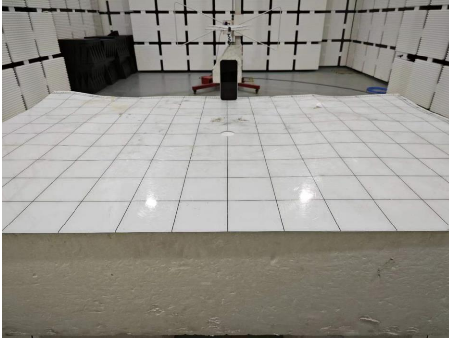
Set-up for Radiated Spurious Emission, Above 1GHz
