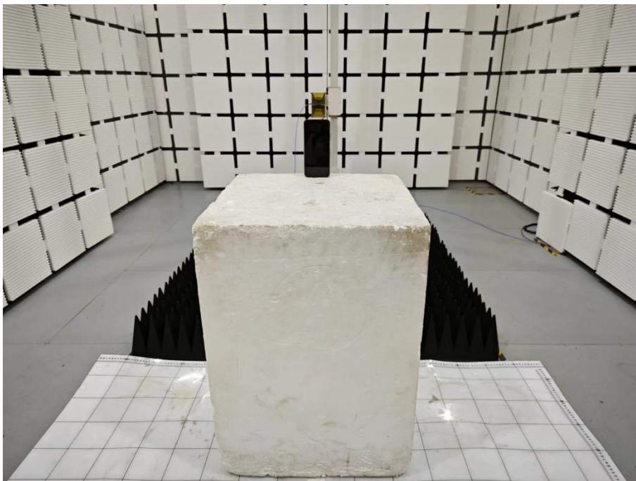
Set-up for Radiated Spurious Emission, Above 1GHz
