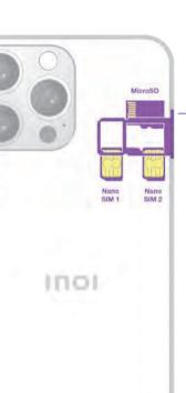
Open the SIM tray with a special key and install one or two Nano SIM cards
