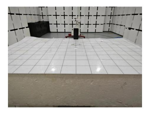
Set-up for Radiated Spurious Emission, Above 1GHz
