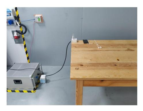
Set-up for Radiated Emission (RE), Below 1GHz
