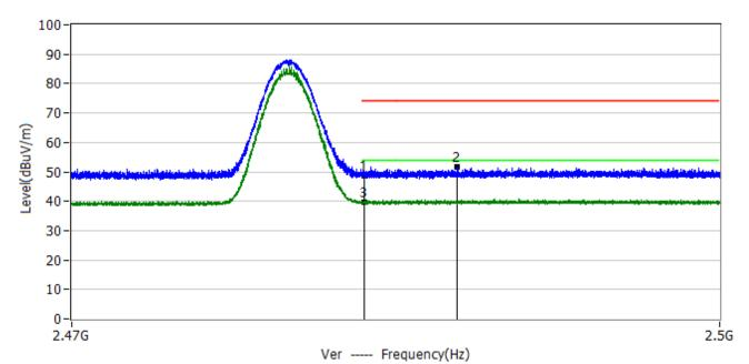
Margin dB -25.20 Reading Factor Level Limit Frequency No. Detector Polar dBu<u>V</u> dB/m dBuV/m dBuV/m2.4835GHz 1\* 14.67 34.13 48.80 74.00 PΚ Ver 2\* 2.4878GHz 17.45 34.14 51.59 74.00 -22.41 PΚ Ver 3\* 2.4835GHz 5.67 34.13 54.00 -14.20 39.80 ΑV Ver
