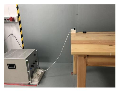
Radiated Spurious Emission Test Setup Photo - Below 1GHz
