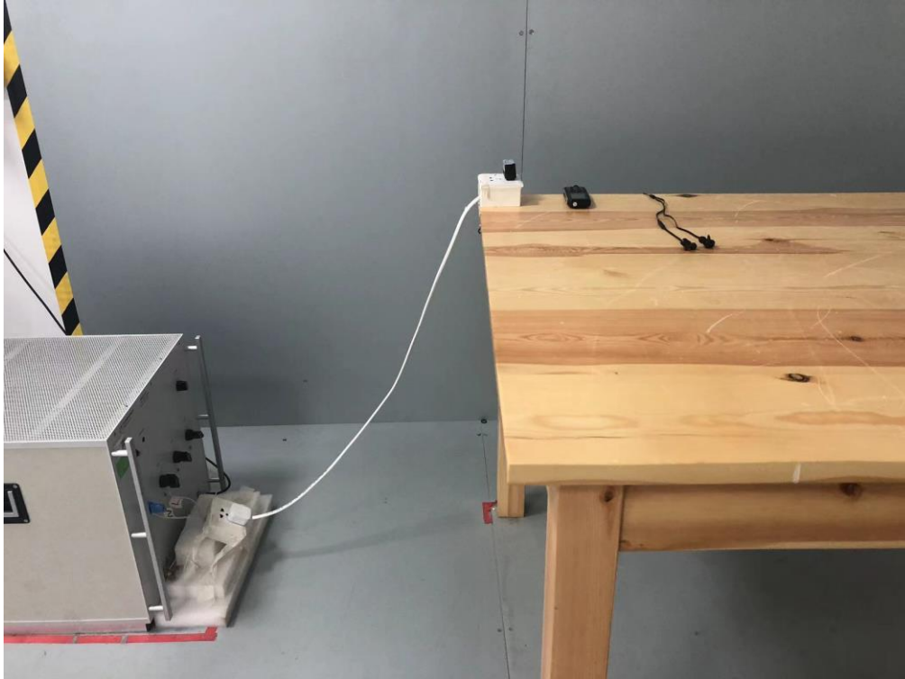
Conducted Emission Test Setup Photo
