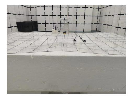
Radiated Emission Test Setup Photo - Above 1GHz
