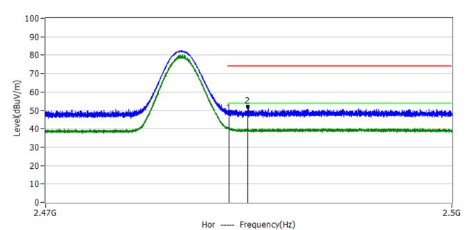
Margin dB -25.60 Reading dBuV Factor Level Limit Frequency No. Detector Polar dB/m 34.13 dBuV/m 74.00 dBuV/m 2.4835GHz 1\* 14.27 48.40 PΚ Hor 2\* 2.4849GHz 17.93 34.13 52.06 74.00 -21.94 PΚ Hor
