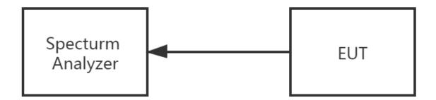
The EUT is connected to the Spectrum Analyzer; the RF load attached to the EUT antenna terminal is 500hm; the path loss as the factor is calibrated to correct the reading. Tune the measurement with the spectrum analyzer's resolution bandwidth (RBW) = 100 kHz. In order to make an accurate measurement, the span is set to be greater than RBW.
