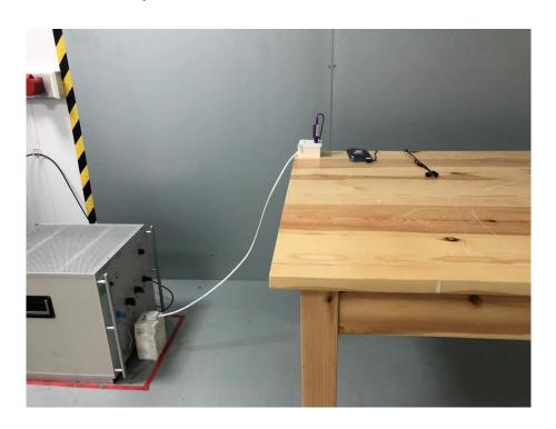
Set-up for Radiated Emission (RE), Below 1GHz
