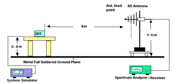
For radiated test from above 1GHz
