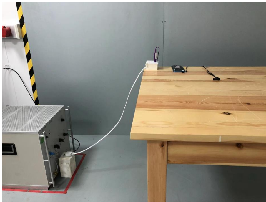
Radiated Emission Test Setup Photo - Below 1GHz
