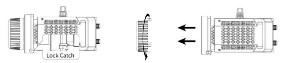
②. When removing the protection cap, press down the lock catch and rotate the protection cap at the same time to take out the protection cap.
