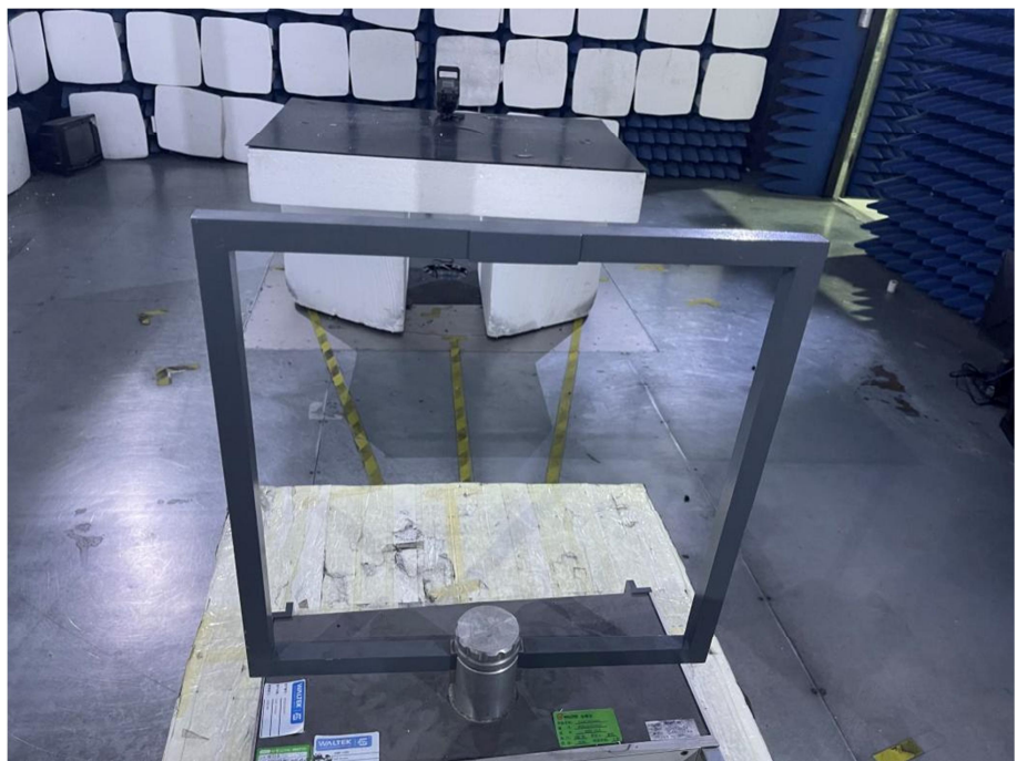
Radiation Emission Test Setup (Below 30MHz)
