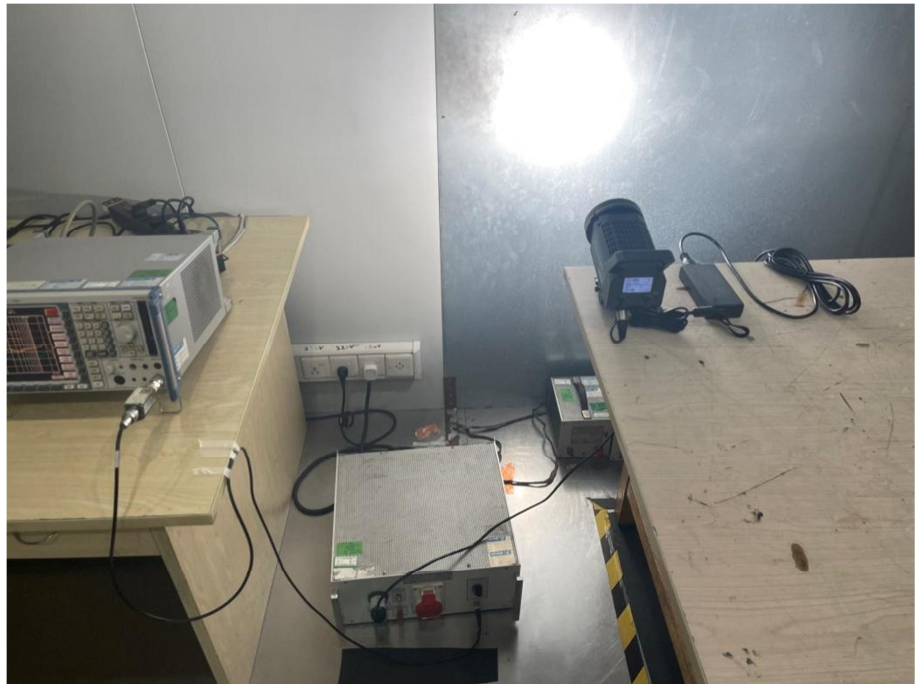
Conducted Emission Test Setup
