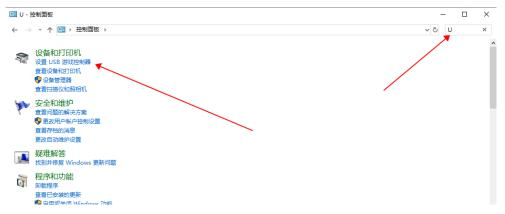
Open the USB game controller and click properties to open the steering wheel test interface.
