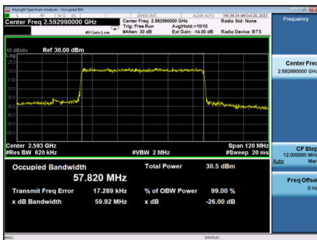
Band n41_60MHz_DFT-s-OFDM_16QAM_ Outer_Full_Mid_CH
