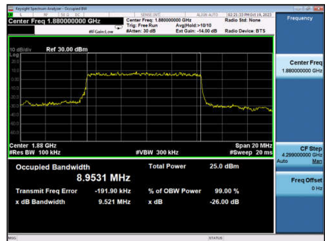
Band n2_10MHz_DFT-s-OFDM_16QAM_ Outer_Full_Mid_CH
