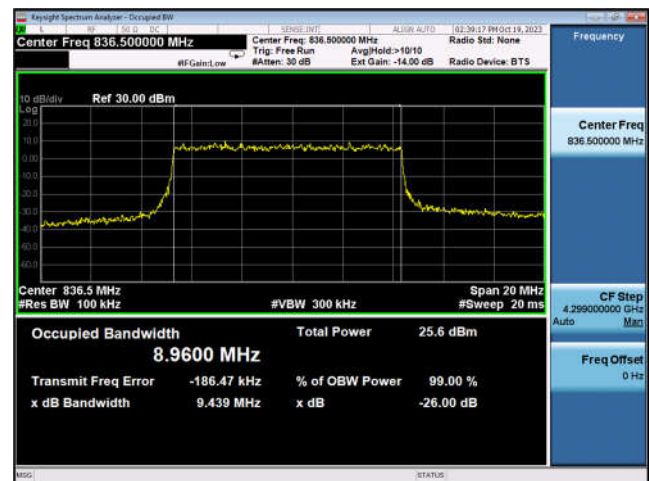
Band n5_10MHz_DFT-s-OFDM_16QAM_ Outer_Full_Mid_CH
