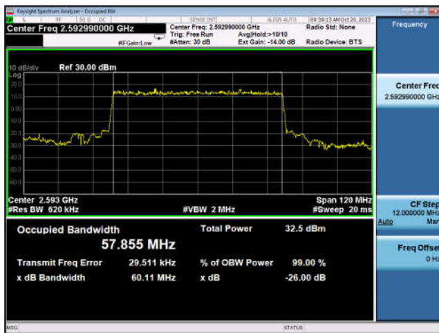
Band n41_60MHz_DFT-s-OFDM_QPSK_ Outer_Full_Mid_CH
