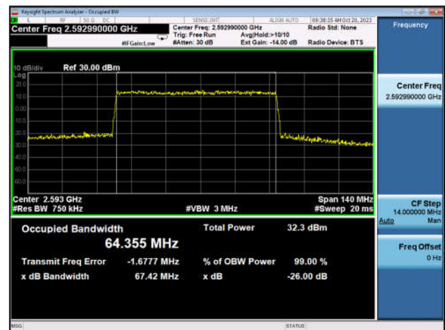
Band n41_70MHz_DFT-s-OFDM_16QAM_ Outer_Full_Mid_CH
