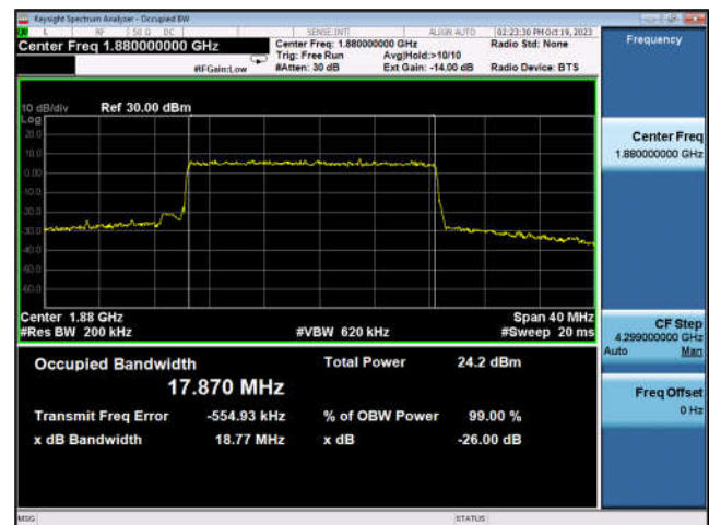
Band n2_20MHz_DFT-s-OFDM_16QAM_ Outer_Full_Mid_CH
