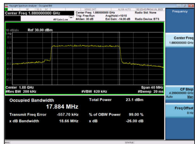
Band n2_20MHz_DFT-s-OFDM_16QAM_ Outer_Full_Mid_CH
