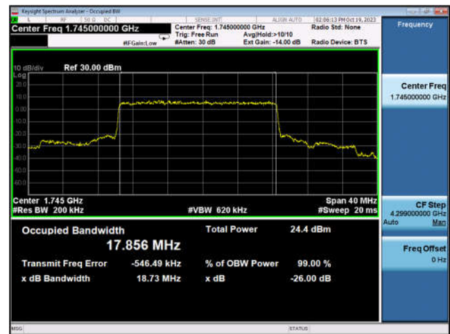
Band n66_20MHz_DFT-s-OFDM_QPSK_ Outer_Full_Mid_CH
