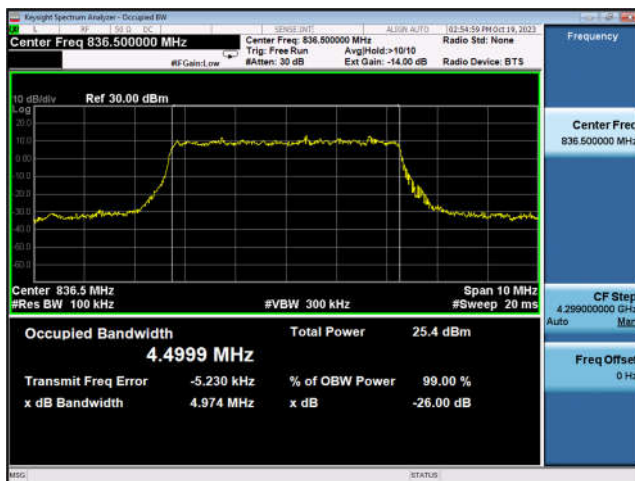
Band n5_5MHz_DFT-s-OFDM_16QAM_ Outer_Full_Mid_CH
