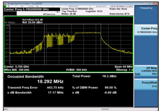
U-NII-3 6dB Bandwidth-802.11ax(20MHz _RU106_2),5825MHz,Ant6
