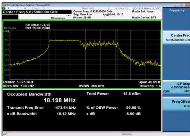
U-NII-3 6dB Bandwidth-802.11ax(20MHz _RU106_1),5825MHz,Ant7
