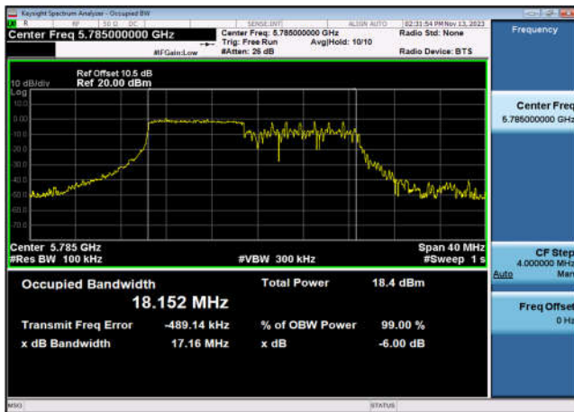
U-NII-3 6dB Bandwidth-802.11ax(20MHz _RU106_1),5825MHz,Ant7
