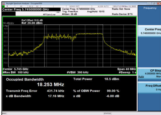
U-NII-3 6dB Bandwidth-802.11ax(20MHz _RU106_2),5785MHz,Ant7
