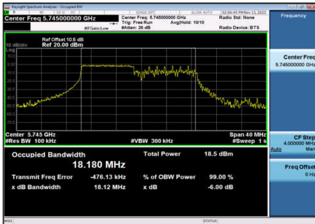
U-NII-3 6dB Bandwidth-802.11ax(20MHz _RU106_1),5785MHz,Ant7
