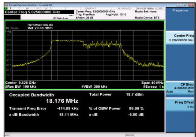
U-NII-3 6dB Bandwidth-802.11ax(20MHz _RU106_1),5825MHz,Ant6
