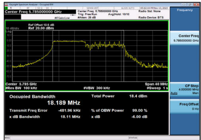
U-NII-3 6dB Bandwidth-802.11ax(20MHz _RU106_1),5825MHz,Ant6
