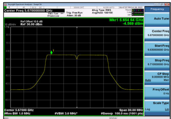
U-NII-2c Power spectral density-802.1 1n(40MHz),5670MHz,Ant6
