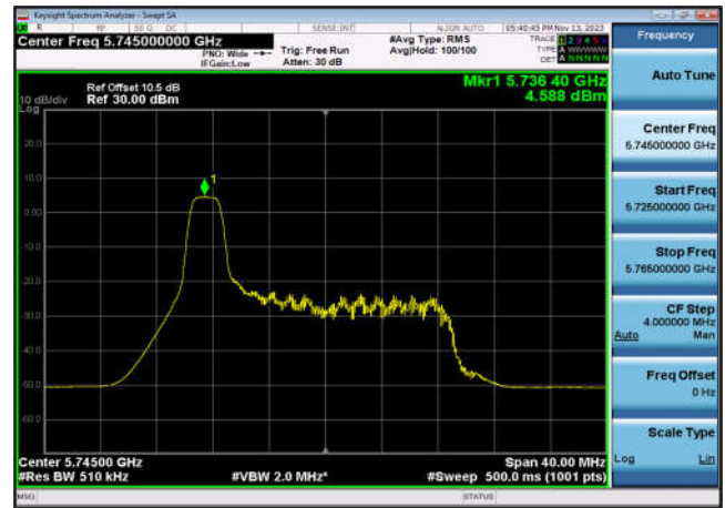
U-NII-3 Power spectral density-802.11 ax(20MHz_RU26_1),5785MHz,Ant6
