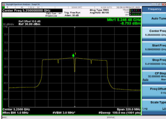
U-NII-2a Power spectral density-802.1 1ac(160MHz),5250MHz,Ant7
