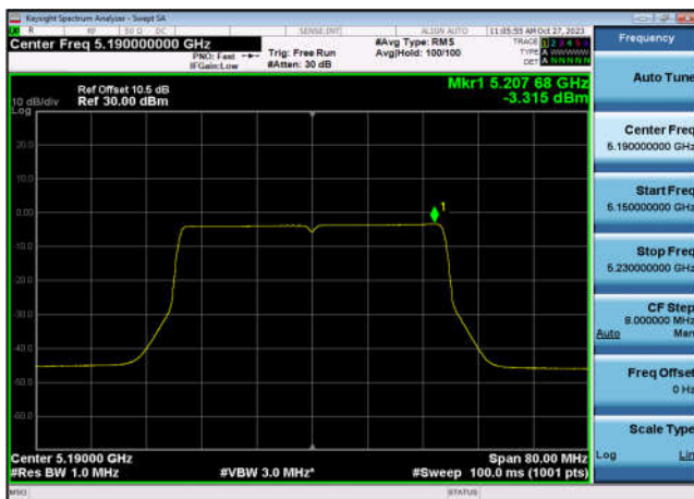
U-NII-1 Power spectral density-802.11 ax(40MHz),5190MHz,Ant7
