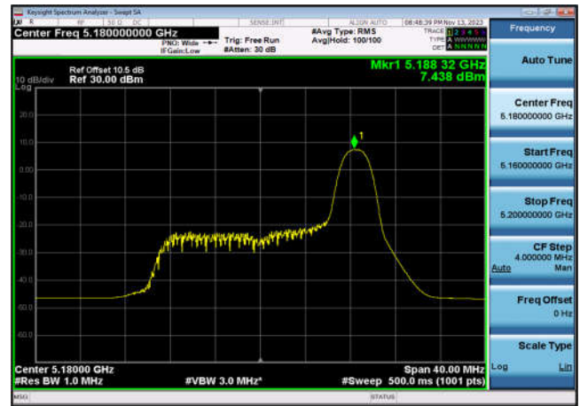
U-NII-1 Power spectral density-802.11 ax(20MHz_RU26_9),5220MHz,Ant6
