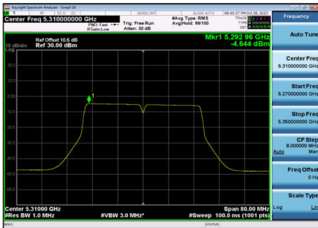
U-NII-2a Power spectral density-802.1 1a(20MHz),5260MHz,Ant7
