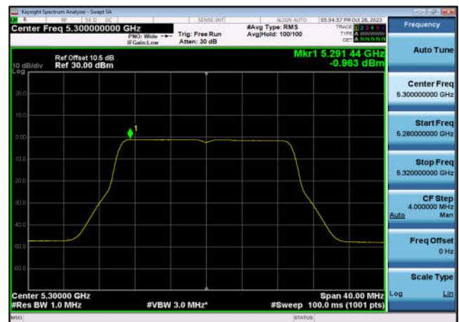
U-NII-2a Power spectral density-802.1 1ax(20MHz),5300MHz,Ant6
