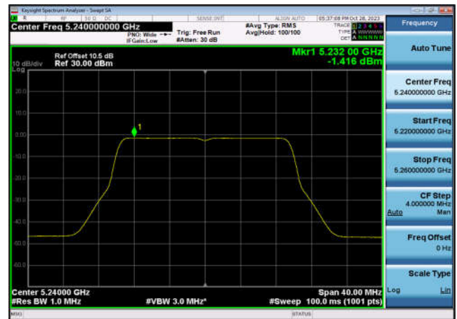
U-NII-1 Power spectral density-802.11 ax(40MHz),5190MHz,Ant6
