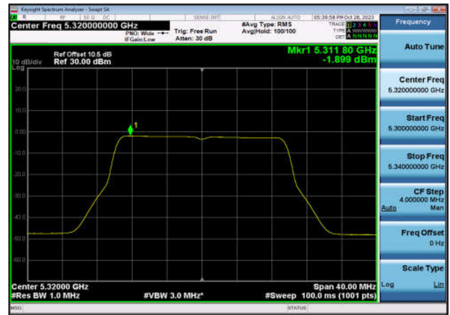
U-NII-2a Power spectral density-802.1 1ax(40MHz),5270MHz,Ant6
