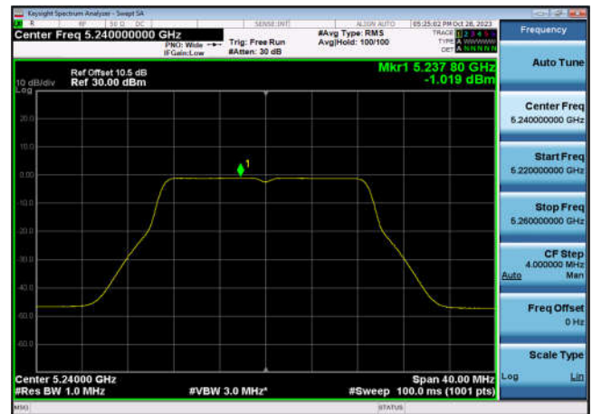
U-NII-1 Power spectral density-802.11 ac(40MHz),5190MHz,Ant6
