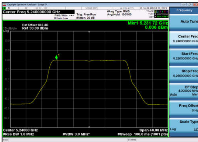
U-NII-1 Power spectral density-802.11 ax(40MHz),5190MHz,Ant7
