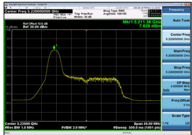
U-NII-1 Power spectral density-802.11 ax(20MHz_RU26_1),5240MHz,Ant6
