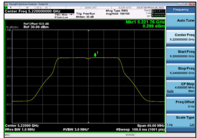
U-NII-1 Power spectral density-802.11 a(20MHz),5240MHz,Ant6
