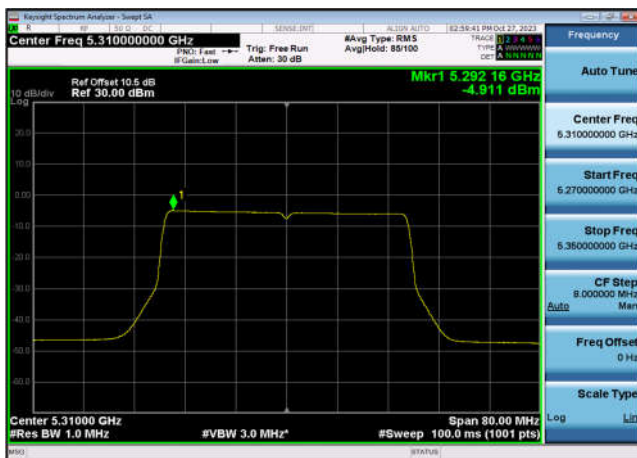
U-NII-2a Power spectral density-802.1 1ax(40MHz),5310MHz,Ant7
