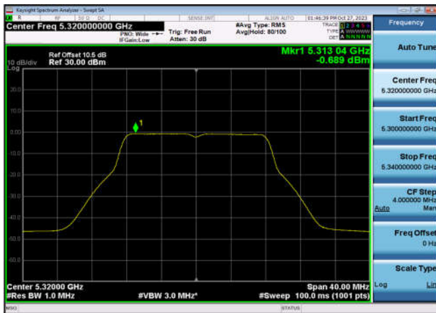
U-NII-2a Power spectral density-802.1 1ac(160MHz),5250MHz,Ant7
