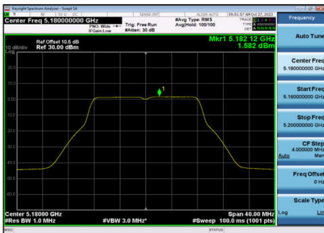
U-NII-1 Power spectral density-802.11 a(20MHz),5180MHz,Ant7
