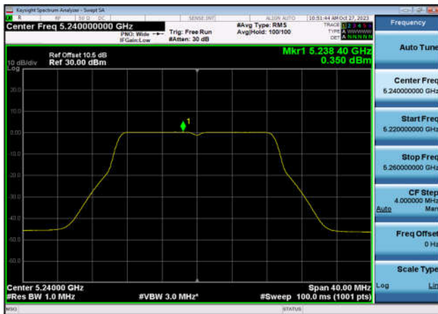
U-NII-1 Power spectral density-802.11 ac(40MHz),5190MHz,Ant7
