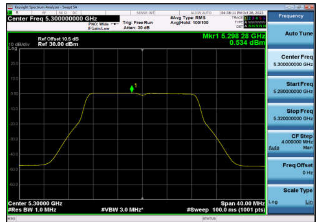
U-NII-2a Power spectral density-802.1 1n(20MHz),5320MHz,Ant6
