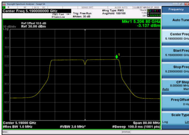
U-NII-1 Power spectral density-802.11 n(40MHz),5230MHz,Ant7
