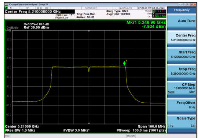
U-NII-1 Power spectral density-802.11 ax(20MHz),5180MHz,Ant6
