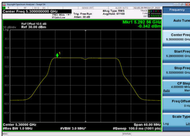
U-NII-2a Power spectral density-802.1 1n(20MHz),5320MHz,Ant7
