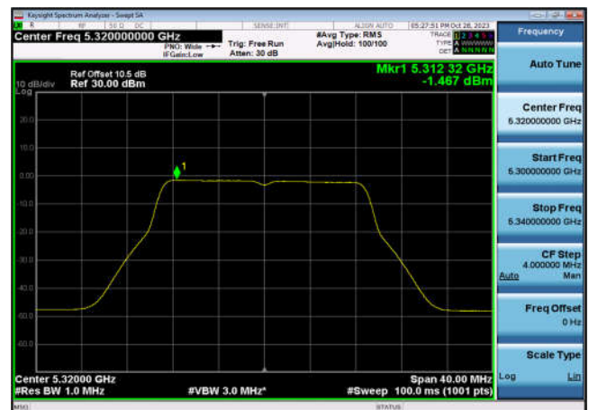
U-NII-2a Power spectral density-802.1 1ac(20MHz),5320MHz,Ant6
