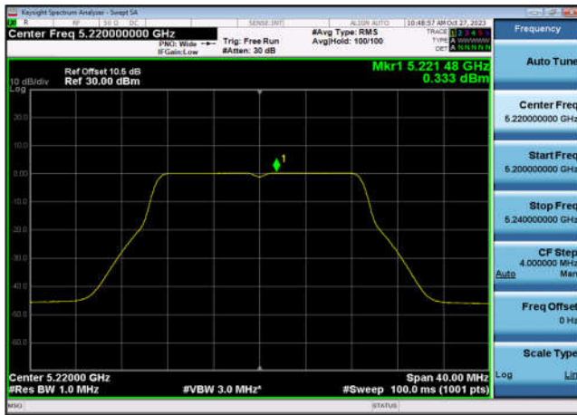
U-NII-1 Power spectral density-802.11 ac(20MHz),5240MHz,Ant7
