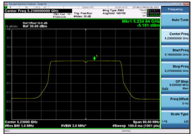
U-NII-1 Power spectral density-802.11 ax(80MHz),5210MHz,Ant6
