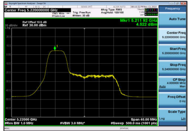
U-NII-1 Power spectral density-802.11 ax(20MHz_RU52_1),5240MHz,Ant6
