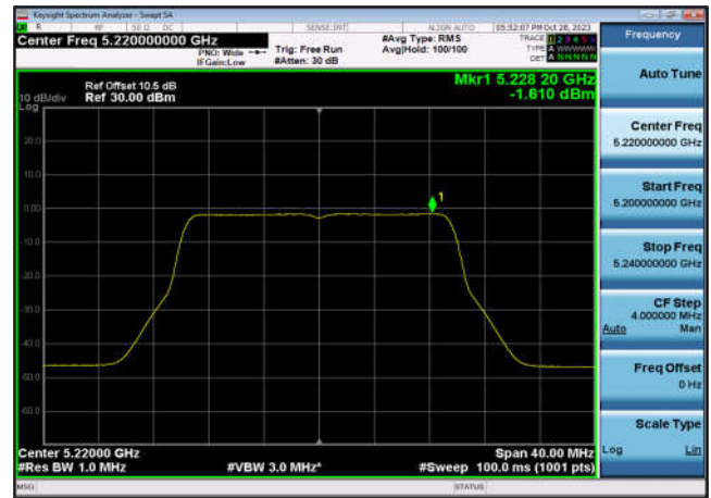
U-NII-1 Power spectral density-802.11 ax(20MHz),5240MHz,Ant6
