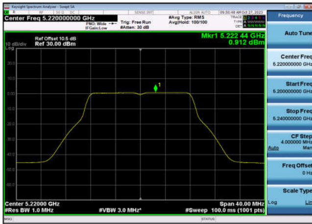
U-NII-1 Power spectral density-802.11 a(20MHz),5240MHz,Ant7
