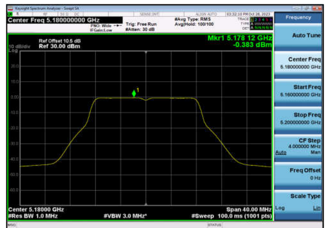
U-NII-1 Power spectral density-802.11 a(20MHz),5180MHz,Ant6
