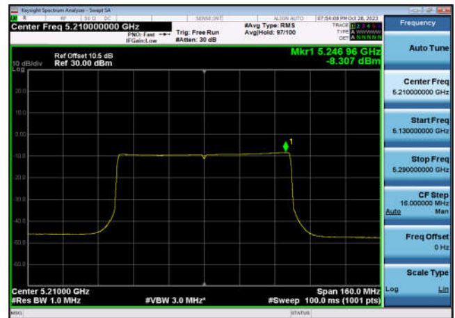
U-NII-1 Power spectral density-802.11 ax(80MHz),5210MHz,Ant6
