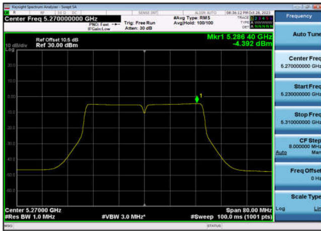
U-NII-2a Power spectral density-802.1 1n(40MHz),5310MHz,Ant7
