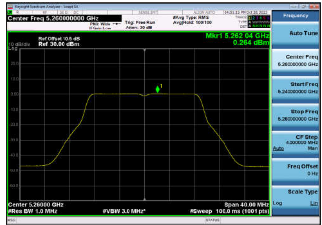
U-NII-2a Power spectral density-802.1 1n(20MHz),5300MHz,Ant6
