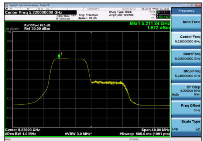
U-NII-1 Power spectral density-802.11 ax(20MHz_RU106_1),5240MHz,Ant6
