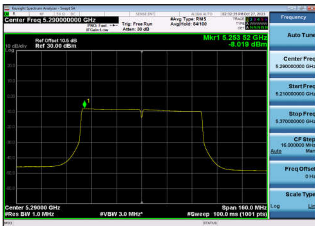
U-NII-2a Power spectral density-802.1 1ac(80MHz),5290MHz,Ant7
