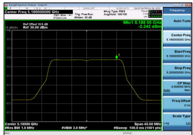
U-NII-1 Power spectral density-802.11 ax(20MHz),5180MHz,Ant6
