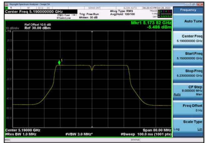
U-NII-1 Power spectral density-802.11 n(40MHz),5230MHz,Ant6
