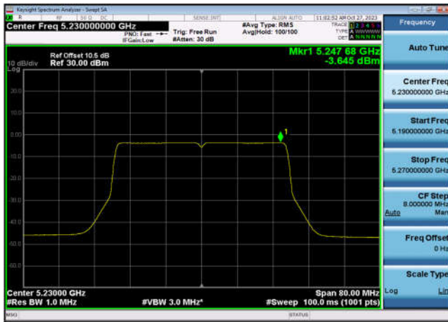
U-NII-1 Power spectral density-802.11 ax(80MHz),5210MHz,Ant7
