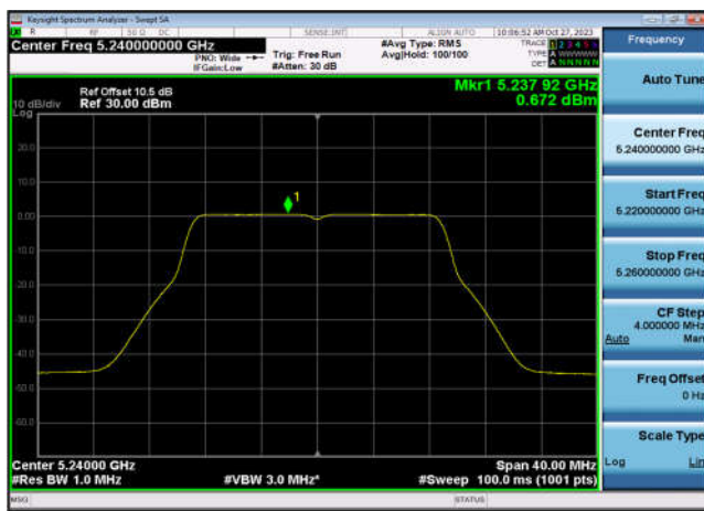
U-NII-1 Power spectral density-802.11 n(20MHz),5240MHz,Ant7
