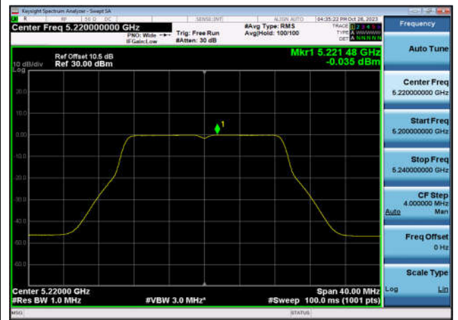
U-NII-1 Power spectral density-802.11 n(20MHz),5240MHz,Ant6
