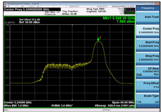
U-NII-1 Power spectral density-802.11 ax(20MHz_RU26_9),5240MHz,Ant6
