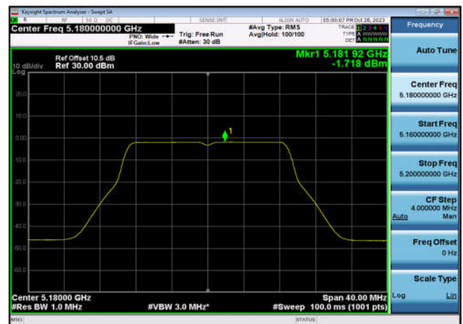
U-NII-1 Power spectral density-802.11 ac(20MHz),5180MHz,Ant6
