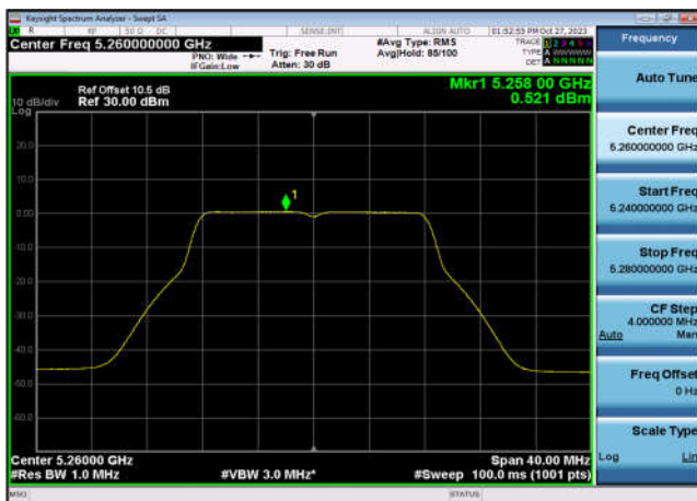
U-NII-2a Power spectral density-802.1 1a(20MHz),5260MHz,Ant7
