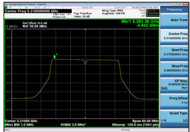
U-NII-2a Power spectral density-802.1 1a(20MHz),5260MHz,Ant6
