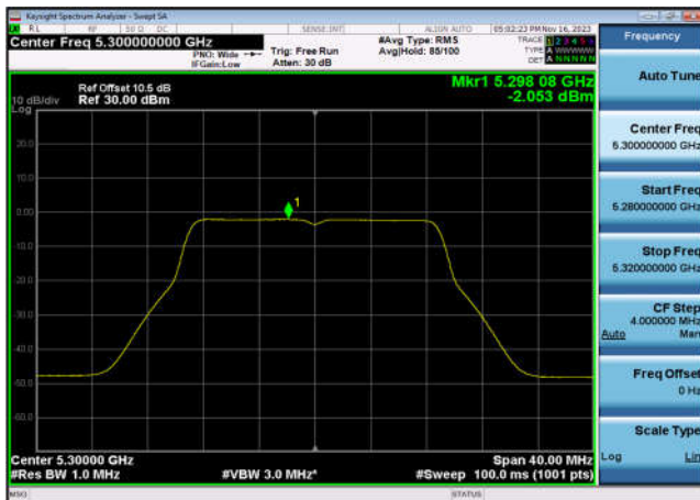
U-NII-2a Power spectral density-802.1 1ac(20MHz),5320MHz,Ant7
