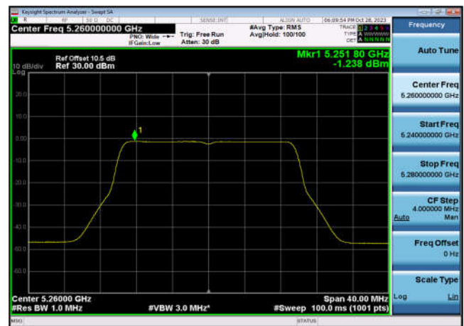
U-NII-2a Power spectral density-802.1 1ax(20MHz),5300MHz,Ant6
