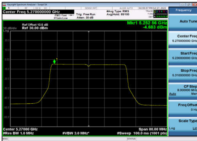
U-NII-2a Power spectral density-802.1 1ax(40MHz),5310MHz,Ant7
