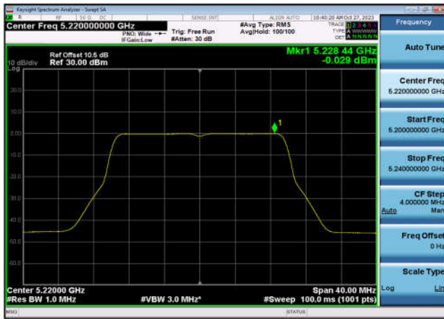
U-NII-1 Power spectral density-802.11 ax(20MHz),5240MHz,Ant7
