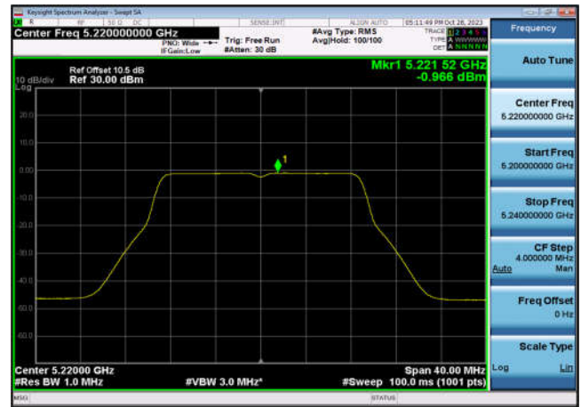
U-NII-1 Power spectral density-802.11 ac(20MHz),5240MHz,Ant6
