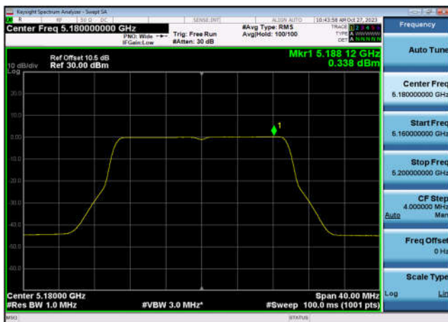
U-NII-1 Power spectral density-802.11 ax(20MHz),5180MHz,Ant7
