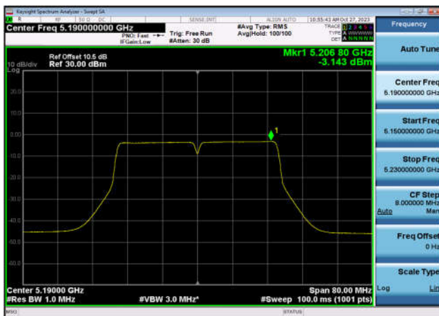
U-NII-1 Power spectral density-802.11 ac(40MHz),5190MHz,Ant7
