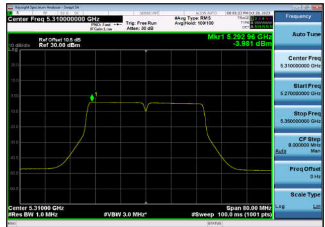
U-NII-2a Power spectral density-802.1 1ac(80MHz),5290MHz,Ant6
