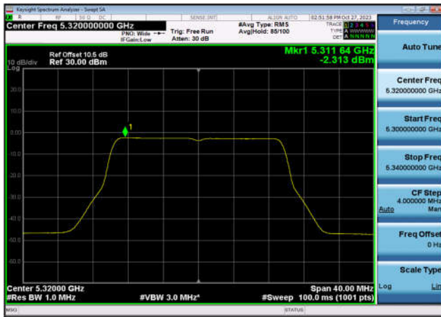
U-NII-2a Power spectral density-802.1 1ax(40MHz),5270MHz,Ant7
