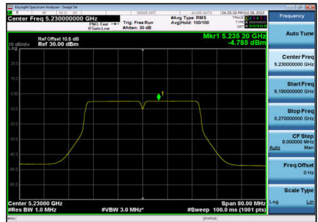
U-NII-1 Power spectral density-802.11 a(20MHz),5180MHz,Ant6
