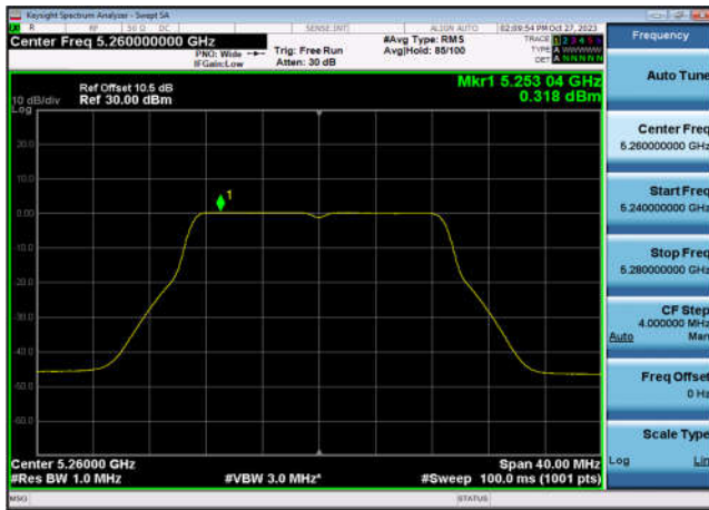
U-NII-2a Power spectral density-802.1 1n(20MHz),5300MHz,Ant7
