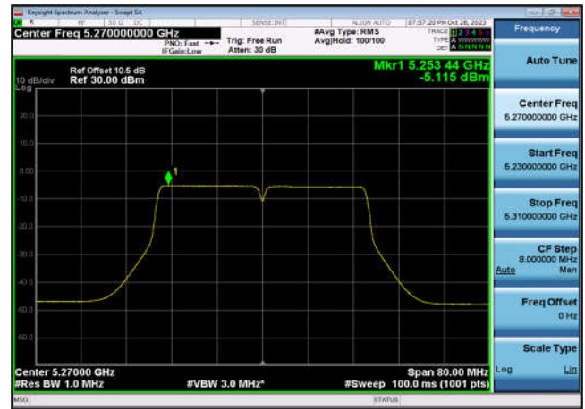
U-NII-2a Power spectral density-802.1 1ac(40MHz),5310MHz,Ant6
