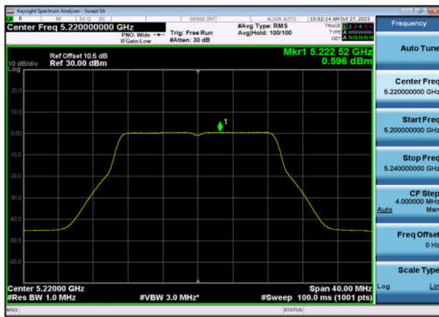
U-NII-1 Power spectral density-802.11 n(20MHz),5240MHz,Ant7
