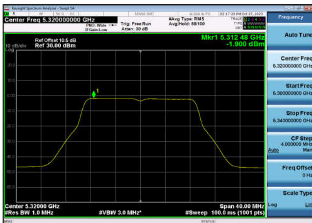
U-NII-2a Power spectral density-802.1 1ac(20MHz),5320MHz,Ant7
