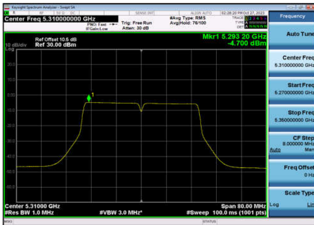
U-NII-2a Power spectral density-802.1 1ac(80MHz),5290MHz,Ant7
