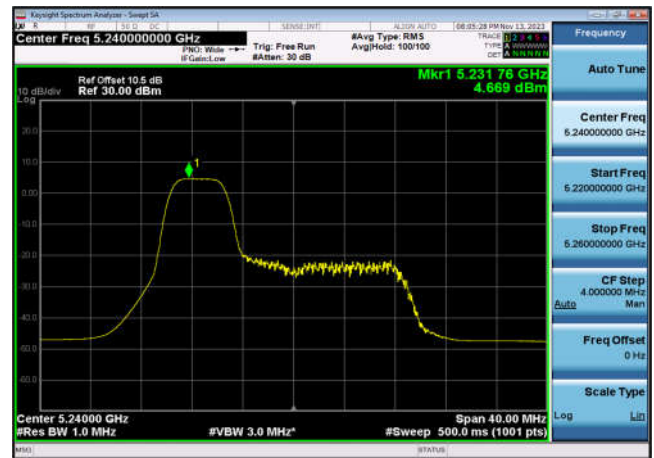
U-NII-1 Power spectral density-802.11 ax(20MHz_RU52_1),5240MHz,Ant6
