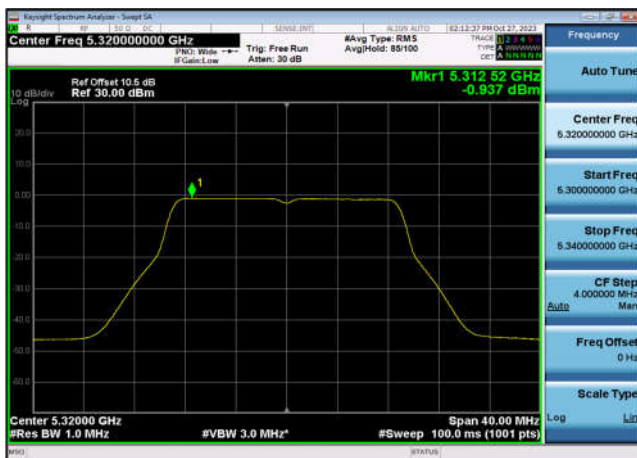
U-NII-2a Power spectral density-802.1 1n(20MHz),5320MHz,Ant7
