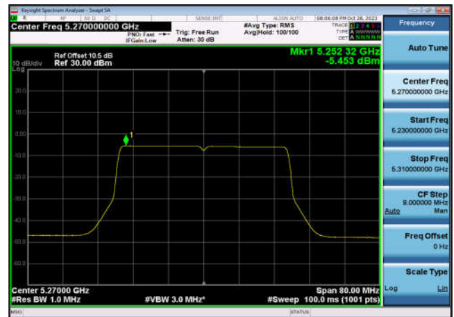
U-NII-2a Power spectral density-802.1 1ax(40MHz),5310MHz,Ant6
