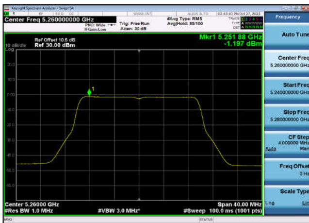
U-NII-2a Power spectral density-802.1 1ax(20MHz),5300MHz,Ant7
