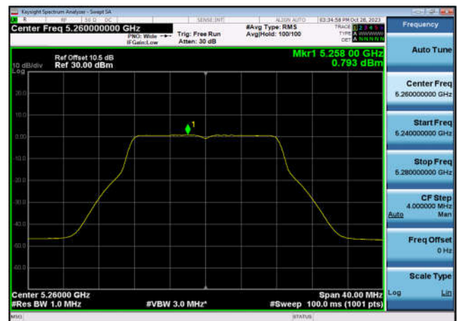
U-NII-2a Power spectral density-802.1 1a(20MHz),5260MHz,Ant6
