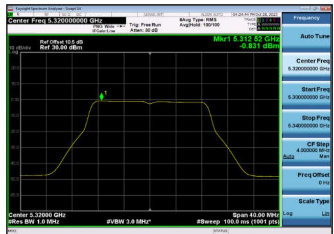
U-NII-2a Power spectral density-802.1 1n(20MHz),5320MHz,Ant6
