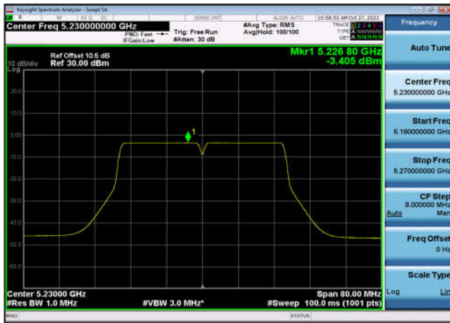
U-NII-1 Power spectral density-802.11 ac(80MHz),5210MHz,Ant7
