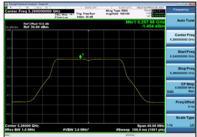
U-NII-2a Power spectral density-802.1 1ac(20MHz),5300MHz,Ant6
