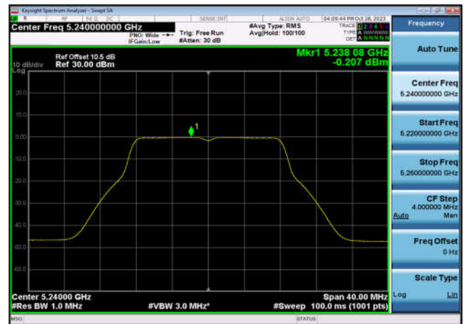
U-NII-1 Power spectral density-802.11 ac(20MHz),5180MHz,Ant6
