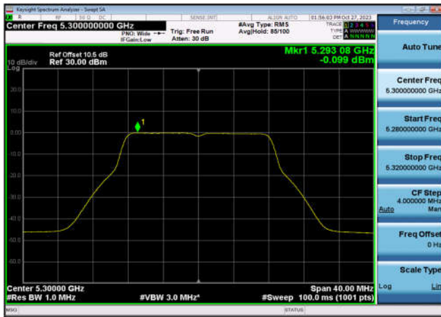
U-NII-2a Power spectral density-802.1 1a(20MHz),5320MHz,Ant7
