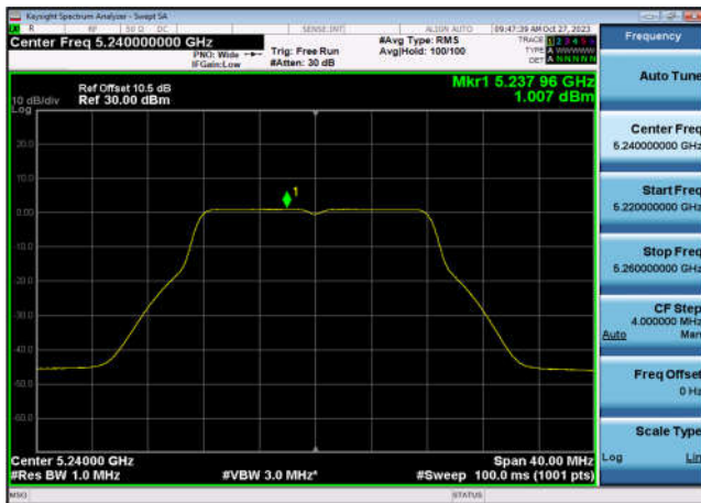
U-NII-1 Power spectral density-802.11 ac(20MHz),5180MHz,Ant7
