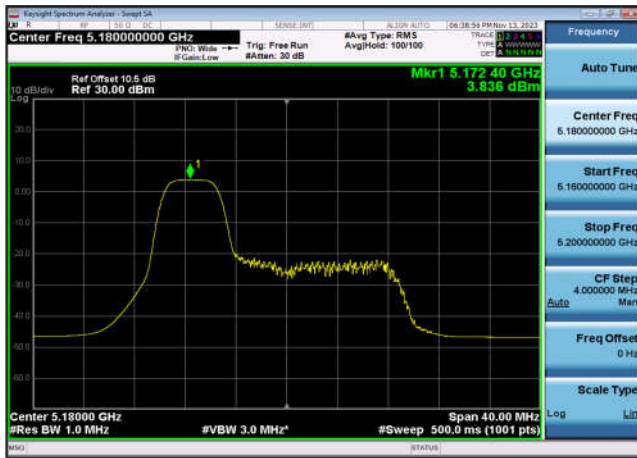
U-NII-1 Power spectral density-802.11 ax(20MHz_RU52_1),5220MHz,Ant7
