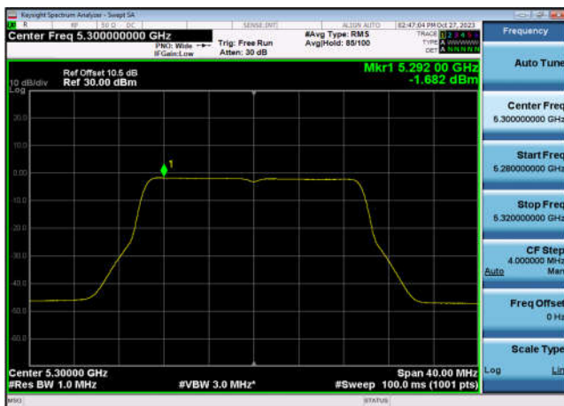
U-NII-2a Power spectral density-802.1 1ax(20MHz),5300MHz,Ant7
