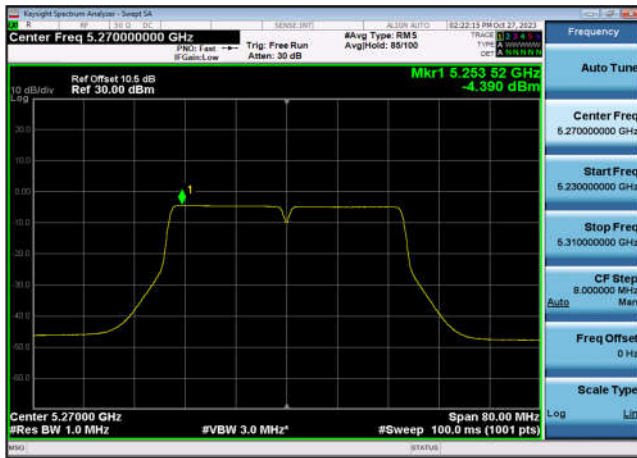
U-NII-2a Power spectral density-802.1 1ac(40MHz),5310MHz,Ant7
