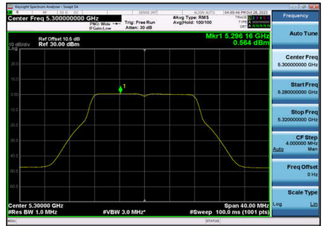
U-NII-2a Power spectral density-802.1 1a(20MHz),5320MHz,Ant6
