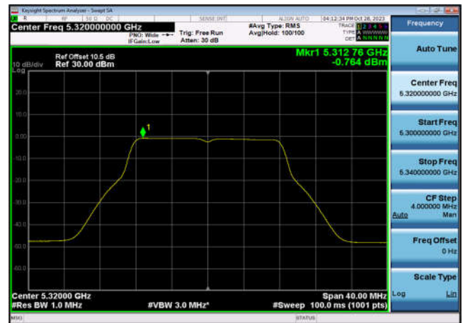
U-NII-2a Power spectral density-802.1 1ac(160MHz),5250MHz,Ant6
