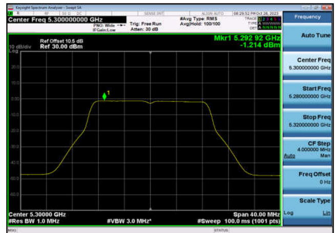
U-NII-2a Power spectral density-802.1 1ac(20MHz),5320MHz,Ant6
