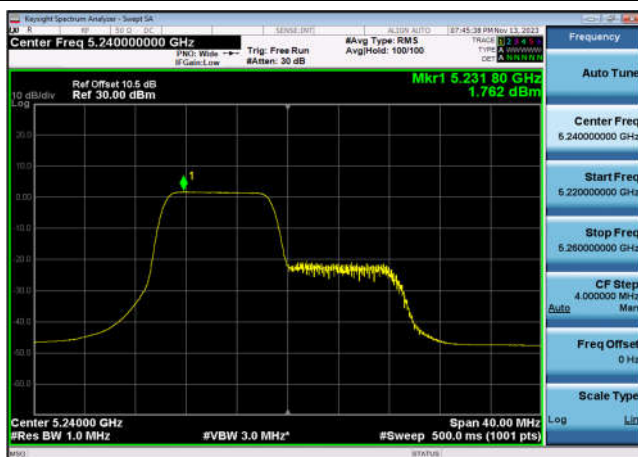
U-NII-1 Power spectral density-802.11 ax(20MHz_RU106_1),5240MHz,Ant7
