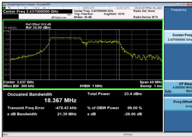
99% Bandwidth-802.11ax(HE20_RU106 _1),2462MHz,Ant7
