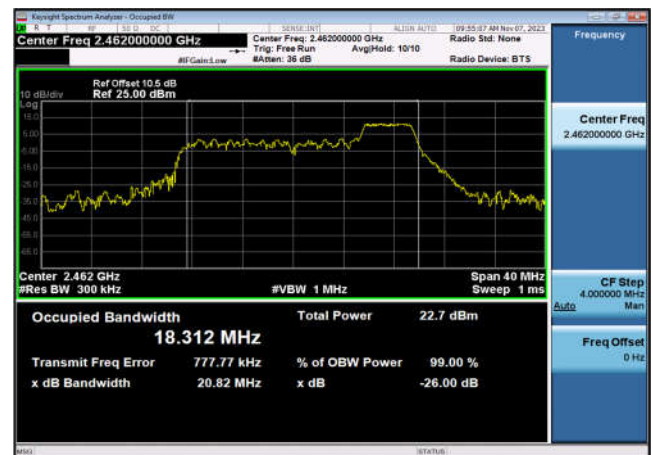
99% Bandwidth-802.11ax(HE20_RU52_4),2462MHz,Ant6
