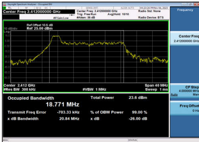
99% Bandwidth-802.11ax(HE20_RU26 _1),2437MHz,Ant7
