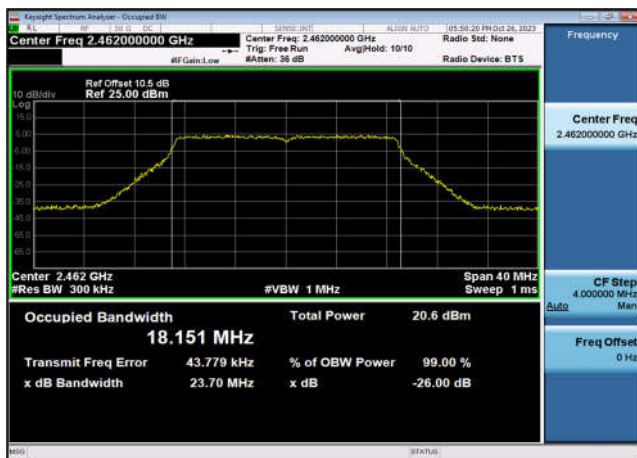
99% Bandwidth-802.11n(HT20),2462MHz ,Ant7
