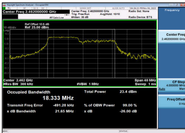
99% Bandwidth-802.11ax(HE20_RU106 _1),2462MHz,Ant7
