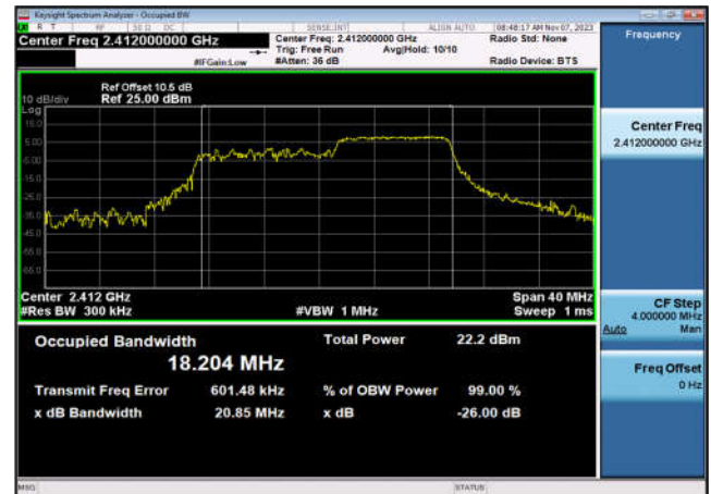
99% Bandwidth-802.11ax(HE20_RU106_2),2437MHz,Ant6
