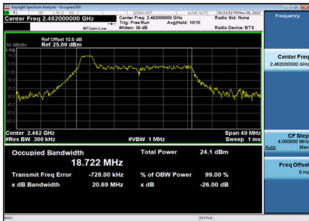
99% Bandwidth-802.11ax(HE20_RU26 _1),2462MHz,Ant7
