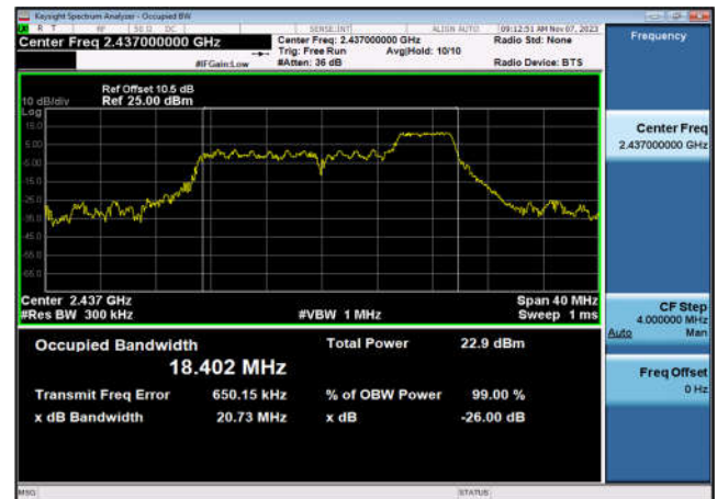
99% Bandwidth-802.11ax(HE20_RU52_4),2462MHz,Ant6
