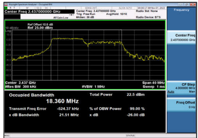
99% Bandwidth-802.11ax(HE20_RU106 _1),2462MHz,Ant6
