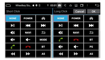
Enter the setting interface to select key learning, "steering wheel control reset" firstly,then long press the buttons on the steering wheel,select the corresponding keys in the interface, When the setting is successful, the corresponding buttons of interface will light up.
