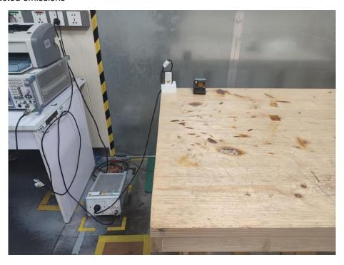
Radiated Measurement Photos 30MHz-1GHz
