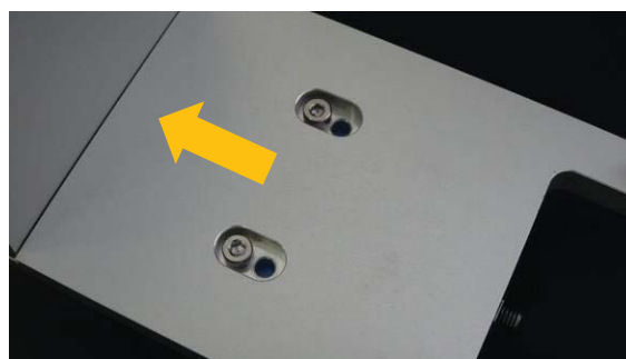
Attaching position for FSR117; rear side of the Force Gauge
