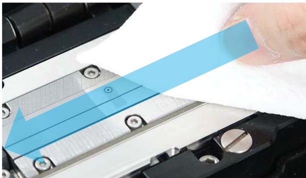
Cleaning of the Recoat mold surface
