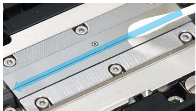
Cleaning of the groove
