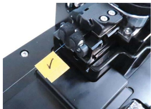
Apply tape to the fiber for marking
