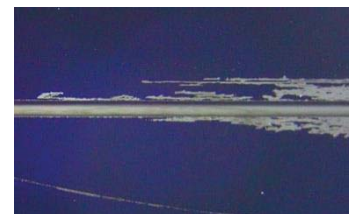
Scratches on the mold surface
