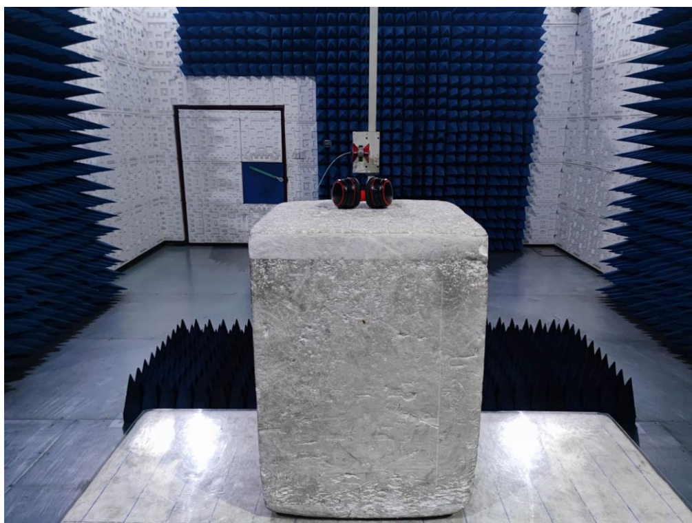
RADIATED EMISSION TEST SETUP ABOVE 1GHz
