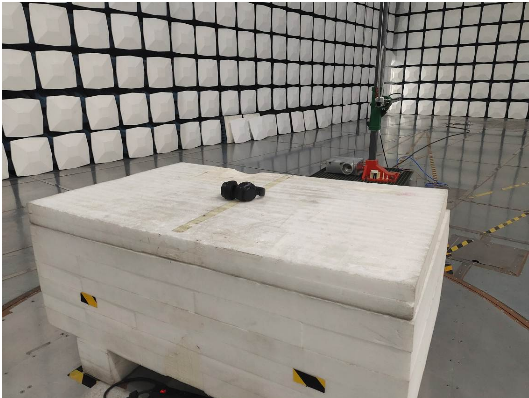
Radiated Emission 9k-30MHz Perpendicular View
