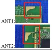
The antenna is Monopole Antenna.
