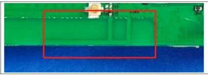
The antenna is PCB antenna.
