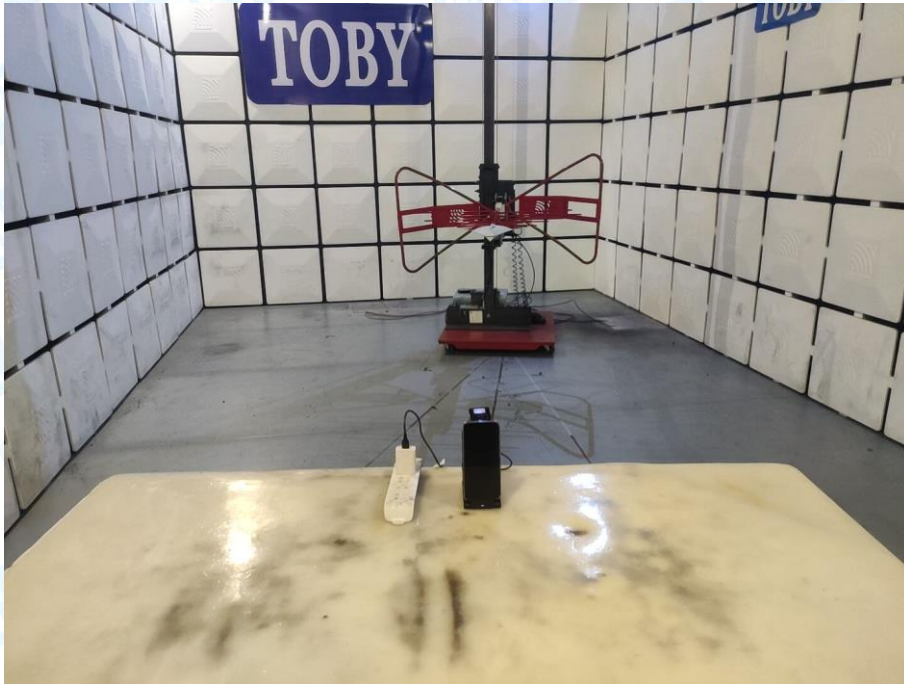
Photo of Setup for Radiated Emission (9KHz-30MHz)
