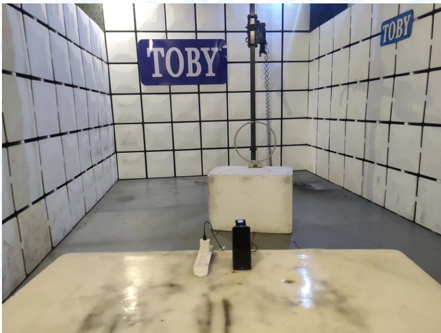
Photo of Setup for Radiated Emission (9KHz-30MHz)
