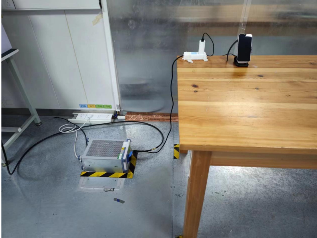
Conducted emission test setup
