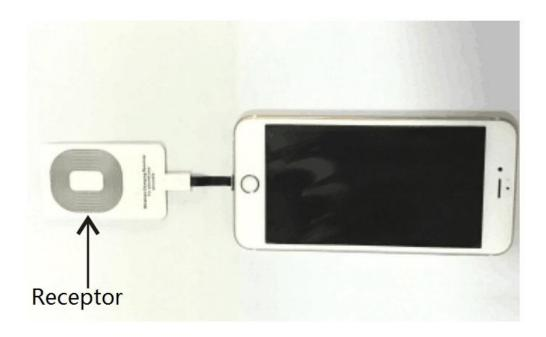
Step 2: Fixed the receptor on the back of the phone.
