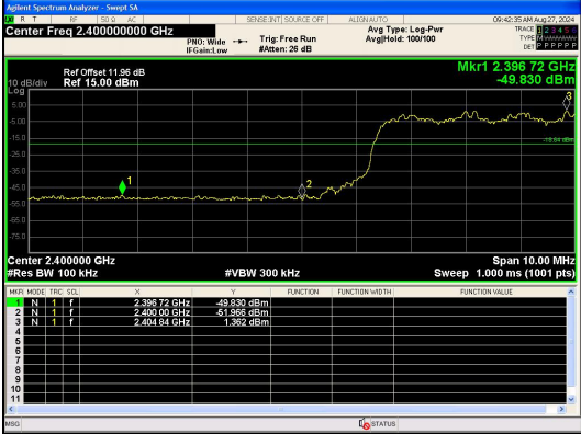
Out Of Band Emission(Left) \pi/4 DQPSK_2-DH5_Channel Hopping
