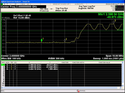
Out Of Band Emission(Left) GFSK_DH5_Channel Hopping
