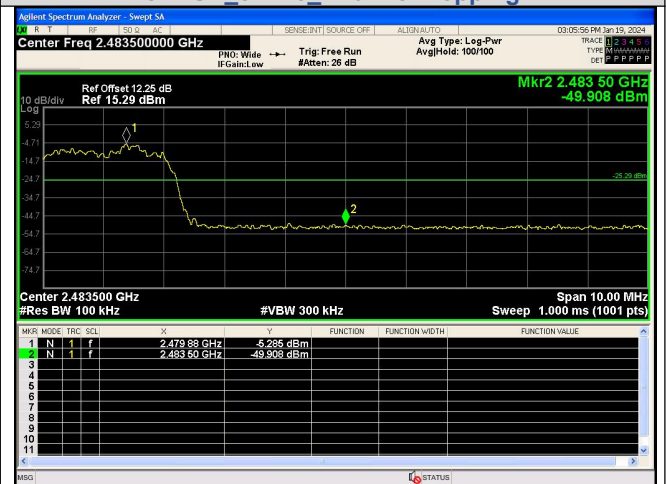
Out Of Band Emission(Right) 8DPSK_3-DH5_Channel Hopping
