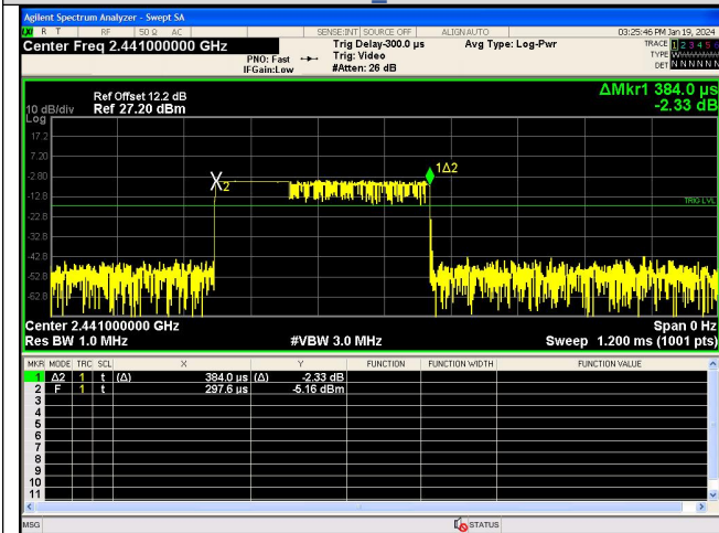
Pulse Width \pi/4 DQPSK_2-DH1
