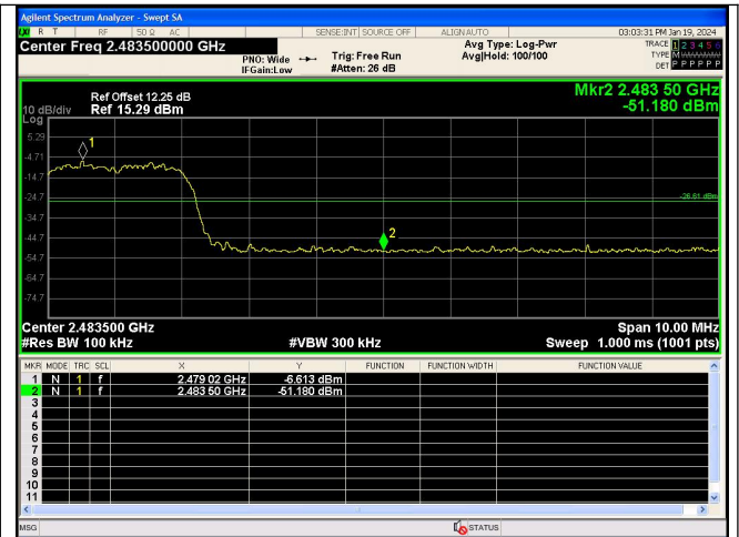
Out Of Band Emission(Right) 8DPSK_3-DH5_Channel Hopping
