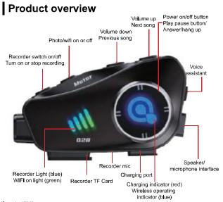
Important Notice: Before installing the headphones, follow the Quick Manual instructions to connect your phone and listen to the sound and volume. If there is a large difference in sound effect and volume after installing it on the helmet, please adjust the position of the speaker in the helmet.
