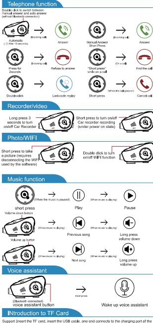
machine, one end connects to the computer, the machine automatically enters the card reader Reader mode: the blue and green lights in the grid alternately slow flash); can be copied or deleted files on the computer Micro SD card (support ≤ 256G)
