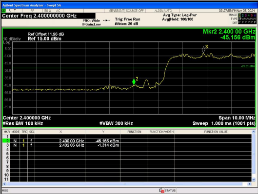
Out Of Band Emission(Left) \pi/4 DQPSK 2-DH5 Channel Hopping
