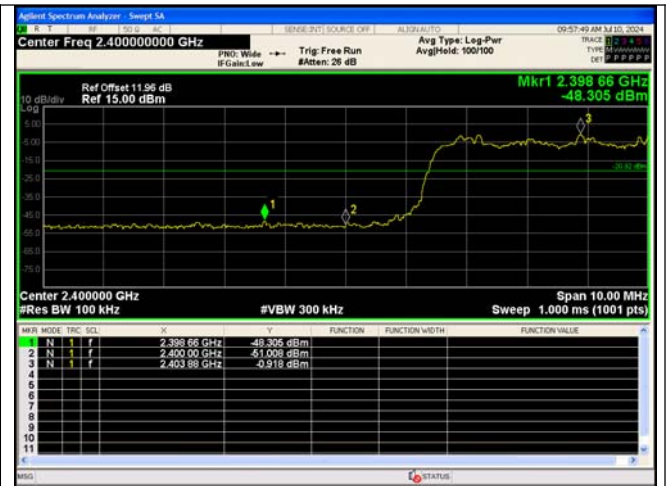
Out Of Band Emission(Left) \pi/4 DQPSK_2-DH5_Channel Hopping
