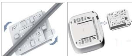
1. Rotate the bracket onto the T-bar of the ceiling.
