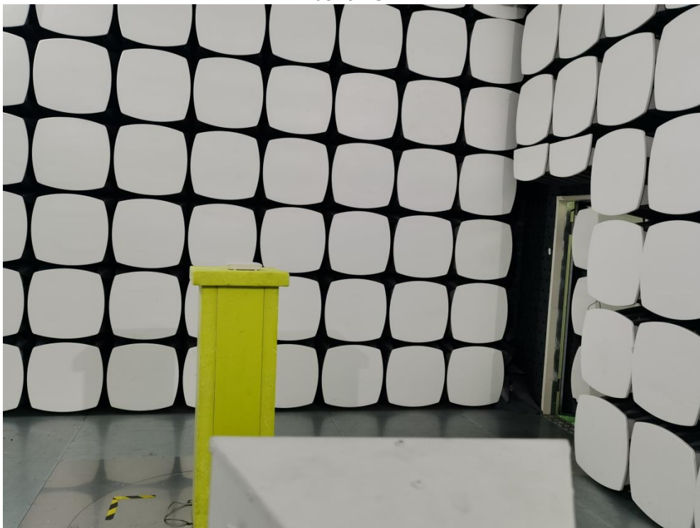
Radiated Emissions Test Photos Above 1GHz
