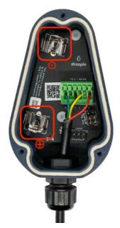
3. Place the battery inside the connectors and make sure that the indicated polarities match the ones from the battery.
