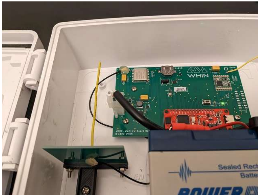
Antenna uFL Connectors Epoxy Glued to Boards
