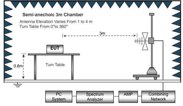
(C) Radiated Emission Test-Up Frequency Above 1GHz
