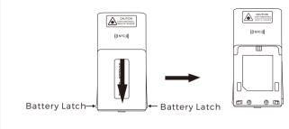
b) Battery Installation: Install the battery in the direction as shown
