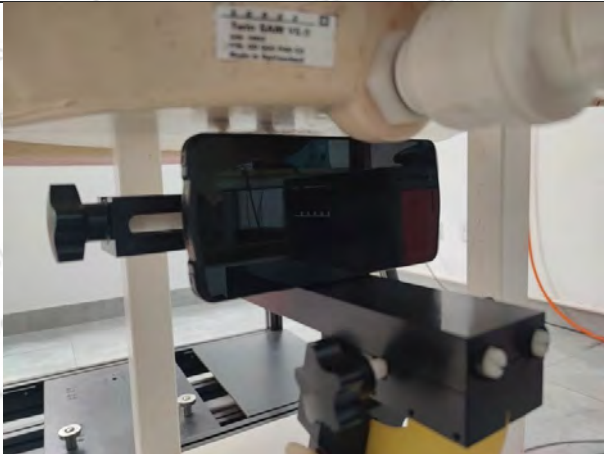
Body-worn Front Side (10mm) Setup Photo
