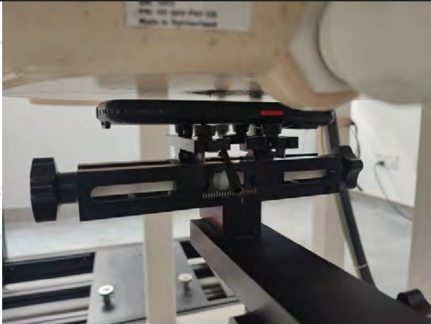
Body-worn Front Side (10mm) Setup Photo
