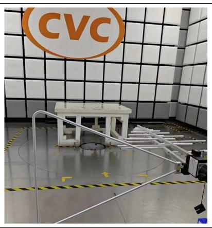
Description: Radiated Emissions/Occupied Channel Bandwidth
